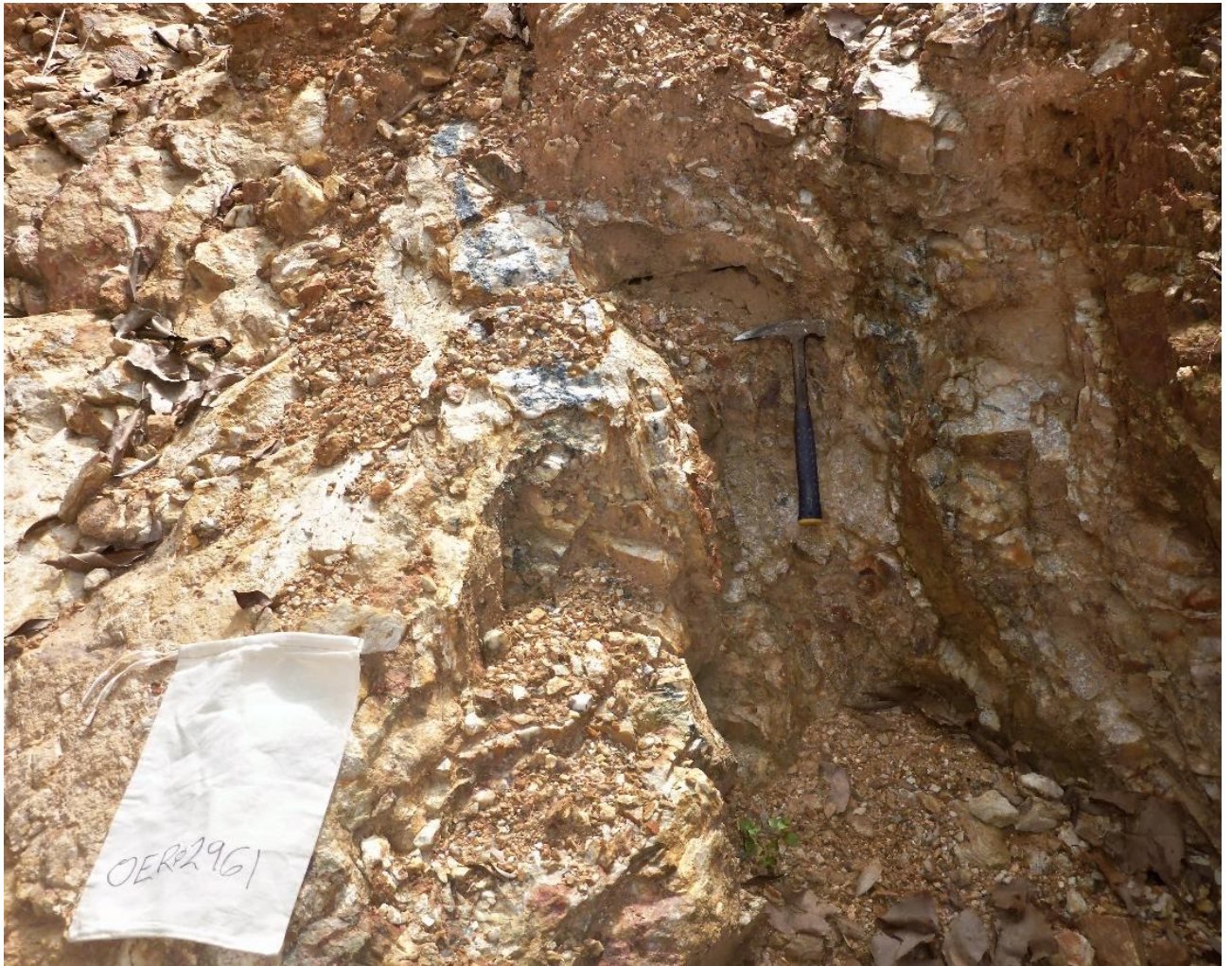
Photo 1: Sample traverse from old costean returned 5.36 Grams per tonne. Sample taken from footwall of laminated quartz vein hosted within weathered sheared felsic intrusive. Alteration appears to be Silica/sericite +/- albite. Galena was observed in some localities.
