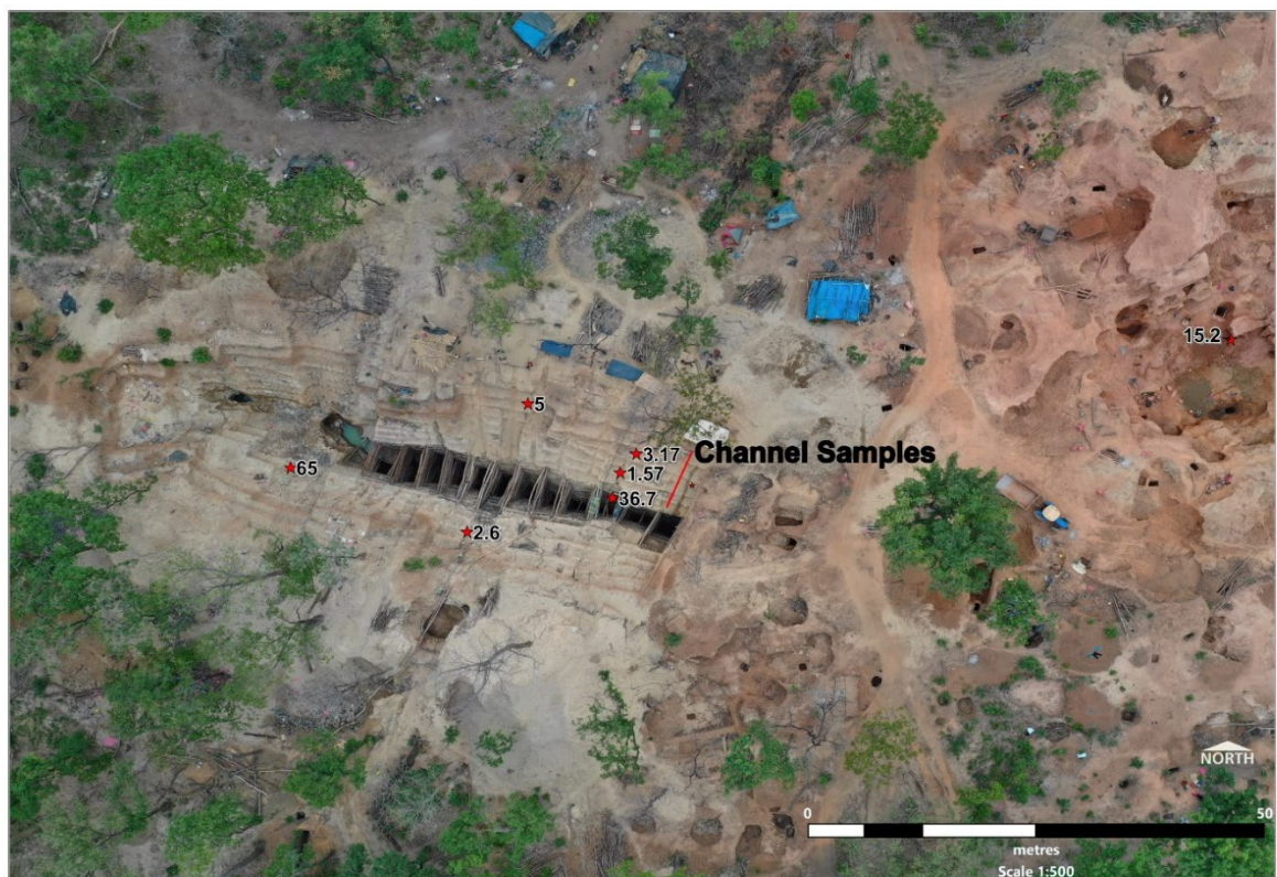
Figure 2: Empire Prospect Gold in Soil Geochemistry over geology. The inset (2b) area is drone photography over the artisanal mining zone showing workings, high grade rock chip samples and the channel sample taken early after commencement of the artisanal mining activity. Figure 3 below depicts the same channel sample.
