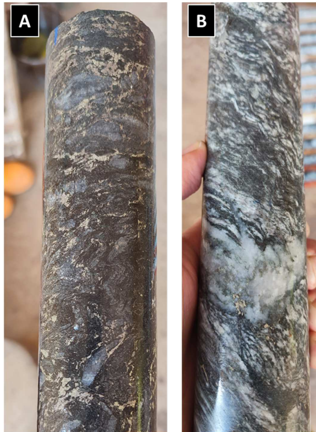
Figure 6: BBM Prospect: - Drill core showing – folded and fractured quartz veins with late pyrrhotite and pyrite mineralization and chlorite alteration in a fracture network [A OEDD-61 50.3m], quartz vein in folded and sheared granite with pyrite and pyrrhotite filling microfractures in quartz [B OEDD-59 75.5m].
