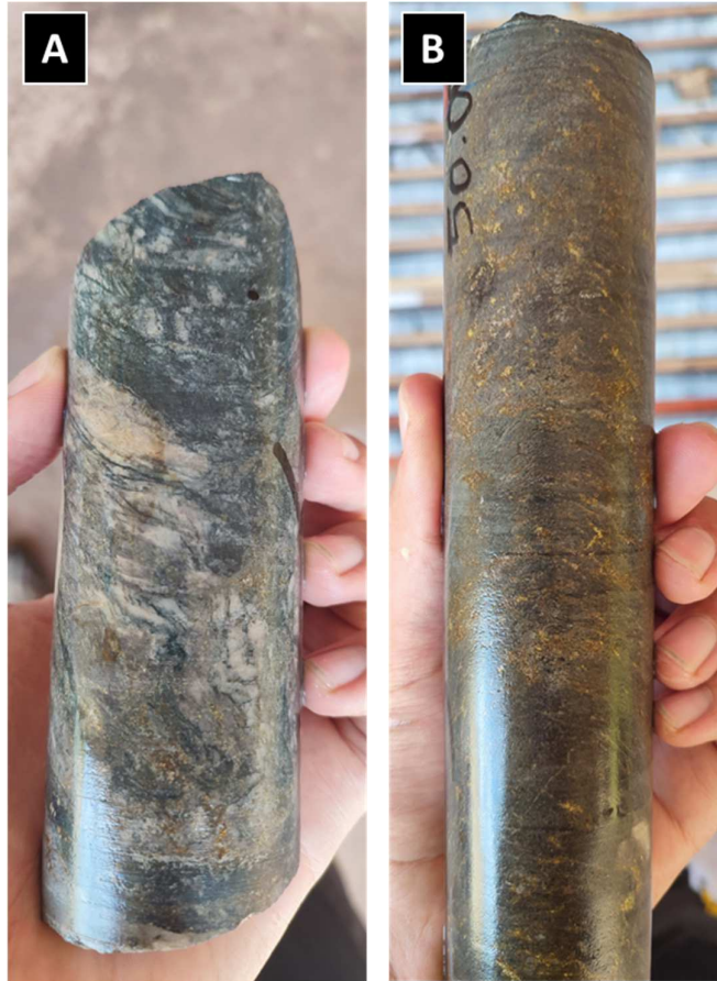
Figure 5: Lando Prospect: - Drill core showing – Disseminated chalcopyrite and pyrite in a brittle/ductile sheared breccia +/- magnetite and chlorite alteration in a fracture network between quartz clasts [A OEDD-47 25.7m], Intense chalcopyrite and pyrite in a fracture network around a fold hinge [B OEDD-47 49.9m].
