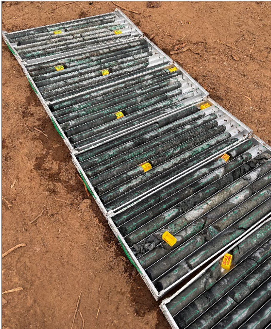
Figure 12-7 Core laid out in the core yard for inspection -BBM, OEDD0152 (source: Bara, 2025)
