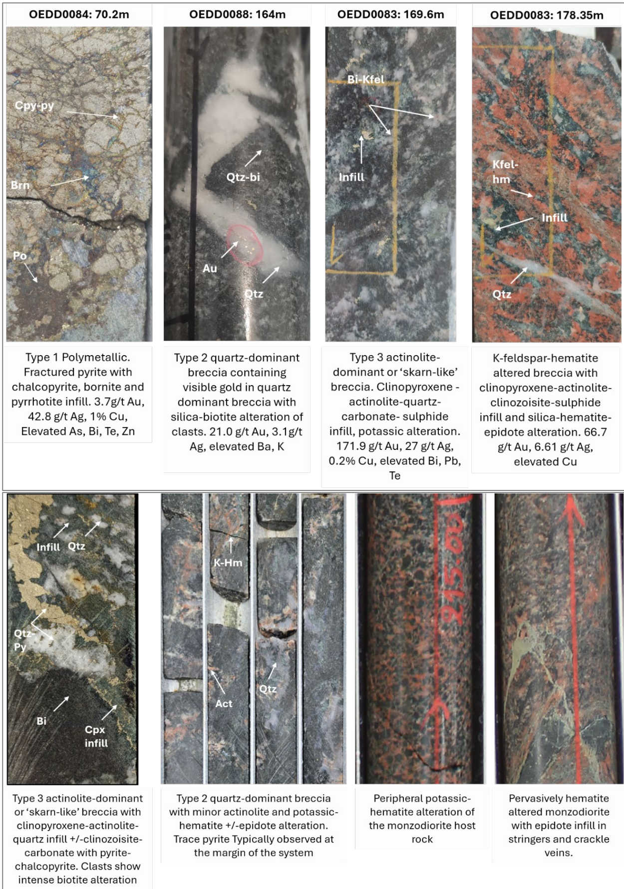
Figure 7-14 Drill core photographs showing different mineralisation and alteration styles at Charger (source: Awalé, 2026)
