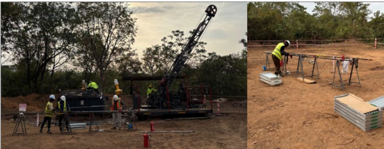
Figure 12-4 BBM drill rig and core mark-up setup (source: Bara, 2025)
